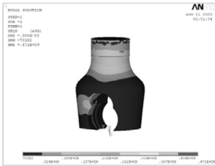
Fig. 16. Stress contour of the optimized top spindle.
